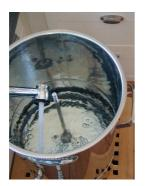
Add 231/531 brewing water – to approx. 2 cm below the upper marking on the tie rod or filling level indicator.
