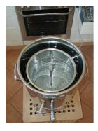
When the mashing-in temperature has been reached a signal tone is emitted; press ENTER to acknowledge. Then insert the malt pipe (with pulled-on seal facing downwards). Ensure that the seal is centred on the malt pipe and sits absolutely flush on the vessel base. Slide in the filter plate to the lower edge (pipe facing up). Then insert the fine sieve (position at bottom of water).
