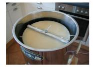
Then press START to continue automatic brewing. Lightly coloured brewing water rises up and spills over. The cycle has begun. The next brewing phases take place fully automatically, as programmed. During some of the brewing phases, the control causes a short pump break to reposition the malt. The display shows the actual and target temperatures as well as the remaining time, which is counted down once the target time has been reached (flashing).
