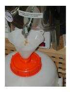
Fill the wort into a sterile 30 l plastic vessel using a funnel (see image) or pipe. First disinfect the vessel and filling aids with sulphuric acid. Do not allow sediment on the base of the vessel to flow out.
